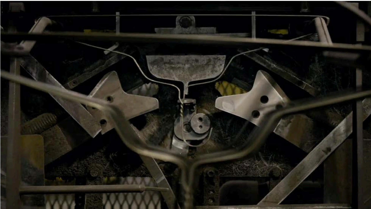
A hanger machine at M&B twists the neck into shape.
