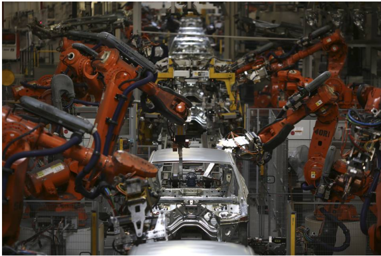
China's economic slowdown could help reduce the cost of steel used by auto makers. Above, robots weld BMW X4 SUV body frames in May at the company's assembly plant in Greer, S.C. PHOTO: LUKE SHARRETT/BLOOMBERG NEWS
